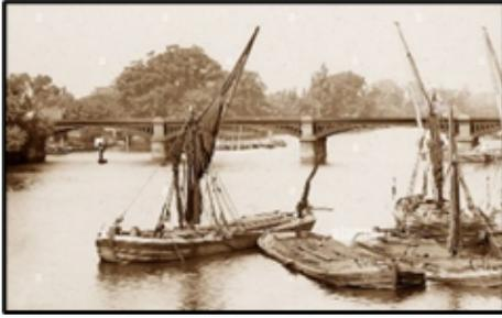
Sailing barges of the early 1800s were entirely open and with no decks. They were small – about 20 tons. Decks then began to be fitted from about 1810.
